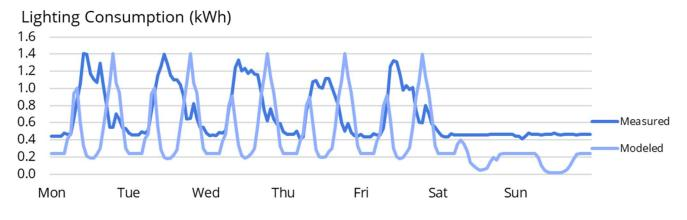
Figure 8 – Average Hourly Lighting Electricity Consumption – Measured (March 2022) vs Modeled (March)
