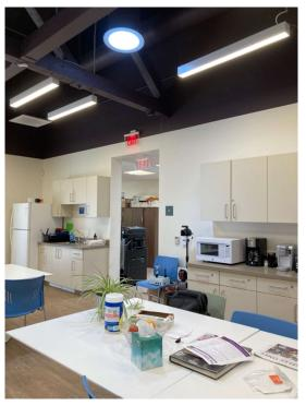
Figure 13 – View of the kitchen area showing visual and thermal comfort measurement apparatuses and one of the TDDs that was in the field of view of the visual comfort measurement.
