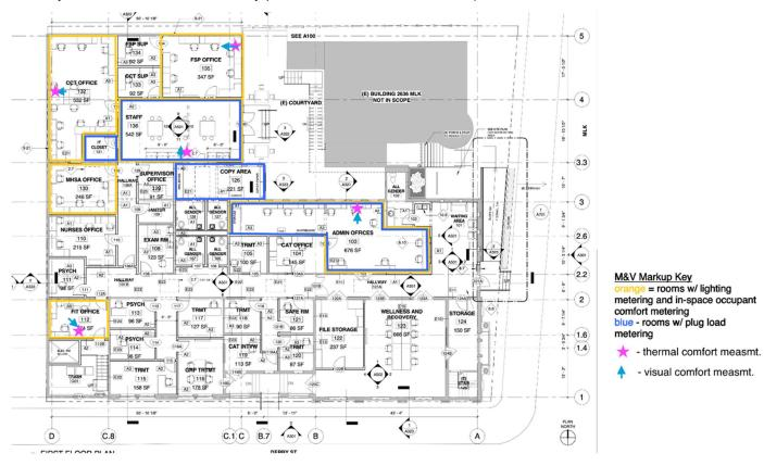
Figure 4 - Locations for visual and thermal comfort spot measurements.
